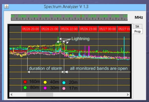
Thunderstorms are very interesting to look at on the RF-Seismograph. The rising air creates a "noise dome" which is usually followed by lightning strikes. After the system passes the noise level drops and propagation improves.
