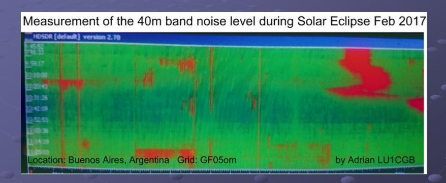
Measurement of the noise level of the partial solar eclipse that occurred in Boenos Aires in February 2017.
