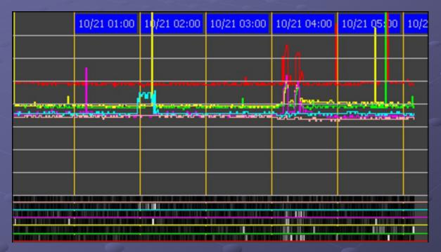
Meteorites can easily be detected by the RF-Seismograph. The start with a fast rise of noise and then peak for about 5 to 10 min., followed by a steep drop back to background noise. As the earth moves though the debris field of meteorites and comets on an annual bases the rate of detected strikes goes up.
