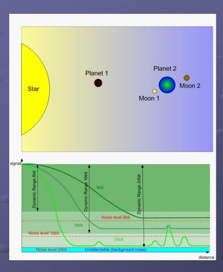
8bit: 256 steps, 4mV step rate @ 1V
