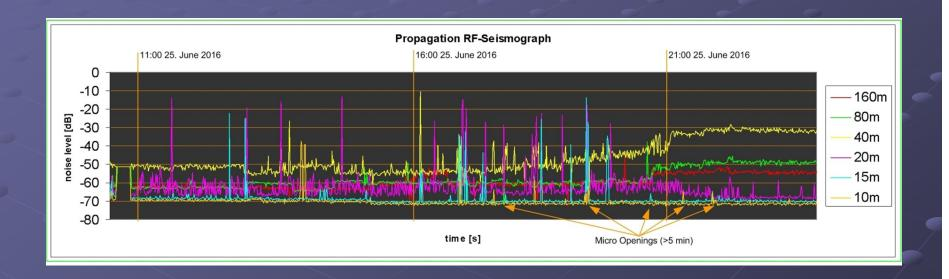
This measurement was done during "Field Day" operations. Located in the North Shore Mountains after the weather turned from sunny to cloudy and then low overcast clouds. Propagation was rendered impossible due to high interference from RF noise created by rising clouds.
