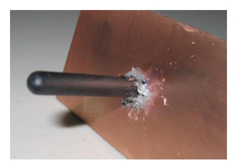
Add sealant to protect coax to dipole transition
