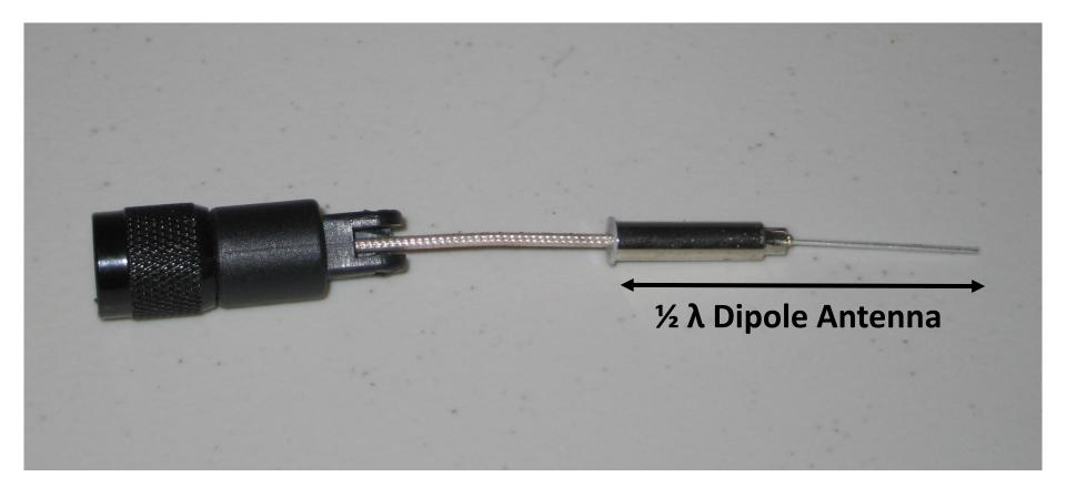
**Optional remove a** portion of the bottom dipole sleeve to expose more feed line
