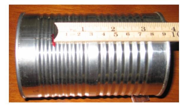
Solder "N" connector with  $\frac{1}{4} \lambda$  probe into hole
