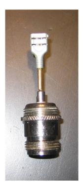
Spade lug added to top of probe to improve return loss per article
