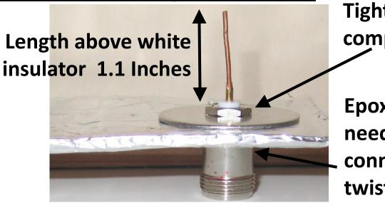
Tighten Nut and compress cardboard
