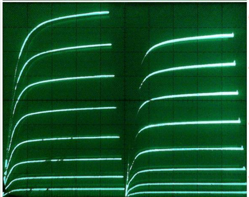
Clockwise from top left: Prototype Tube Matching Adapter on an EICO 667 Tube Tester; 6AU6A pentode curves displayed in the upper and lower storage halves of the 577 -D1 Storage Curve Tracer; Same curves displayed side by side ; Same curves displayed full screen and superimposed on each other . Settings: Horizontal: 50V / Div.; Grid: 1 V / Step; Screen: 200V, Vertical: 10mA / Div. upper right photo, 5 mA / Div. lower left and lower right photos.
