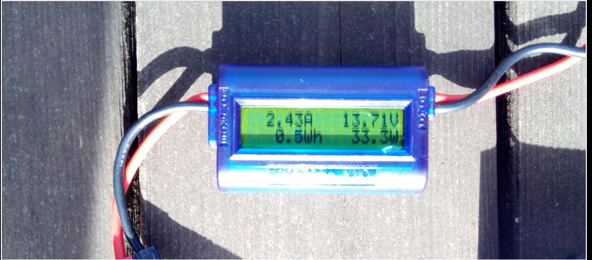
INLINE METER READING, LATE AFTERNOON "SUN WITH SOME CLOUDS", (RC ELECTRONICS WATTS UP METER), YOU ADD THE ANDERSON CONNECTORS
