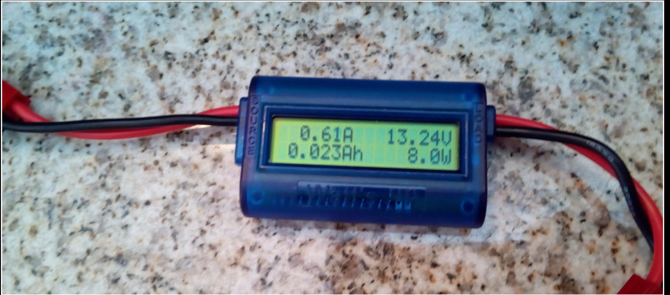
WATT'S UP INLINE METER DISPLAYS CURRENT, VOLTAGE AND WATTS + A ROTATING VALUE DISPLAY IN THE LOWER LEFT CORNER
