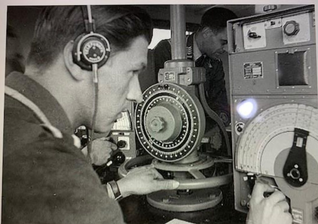
Inside a mobile RP2a station. The dial on the right is the frequency-selector. The operator's hand is on the wheel that rotates the antenna until he hears the signal die. He can then read off the bearing from the scale above the wheel.
