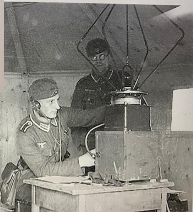
An Fu.NP.E RDF set being operated from a fixed base. Note the shape of the antenna.
